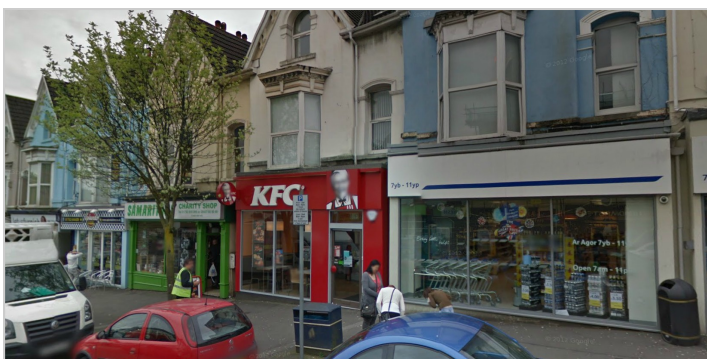
Left: This row of shops shows how fascia signs can be staggered/stepped to provide a relatively uniform transition along a terrace of shops on a sloping street/hill.
